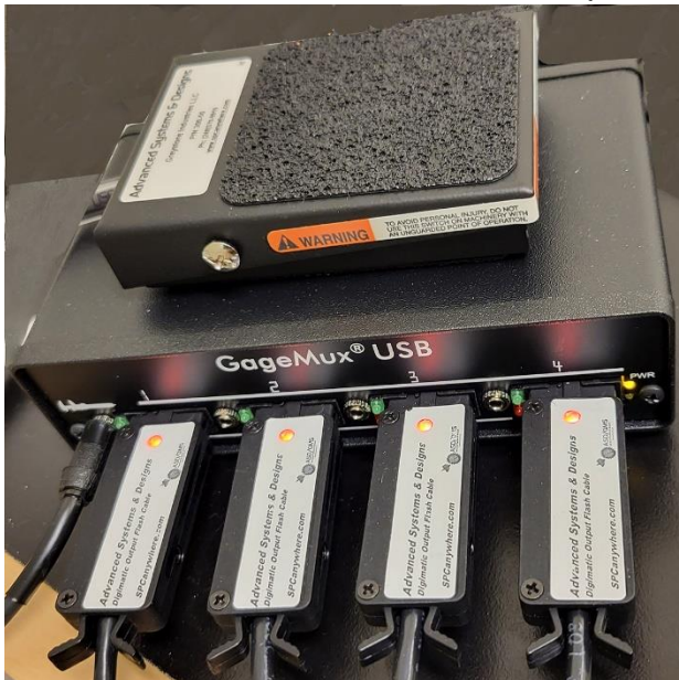
Figure 9. GageMux USB with foot pedal to trigger readings and 4 USB connections to read the 4 balances. Data are dumped into and Excel file on a connected laptop.
